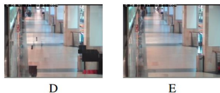
Figure 4: Examples from two VISOR and two CAVIAR videos: (A,B) two random frames, (C) Estimated background using the median filter, (D) using the DCT based method of Reddy et al. ([14]), (E) Our proposed enhanced method
