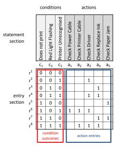
Fig. 4. A decision table example, showing a hypothetical troubleshooting checklist for solving printing failures. Note that we use a vertical layout, which is more suitable when dealing with a large number of conditions.
