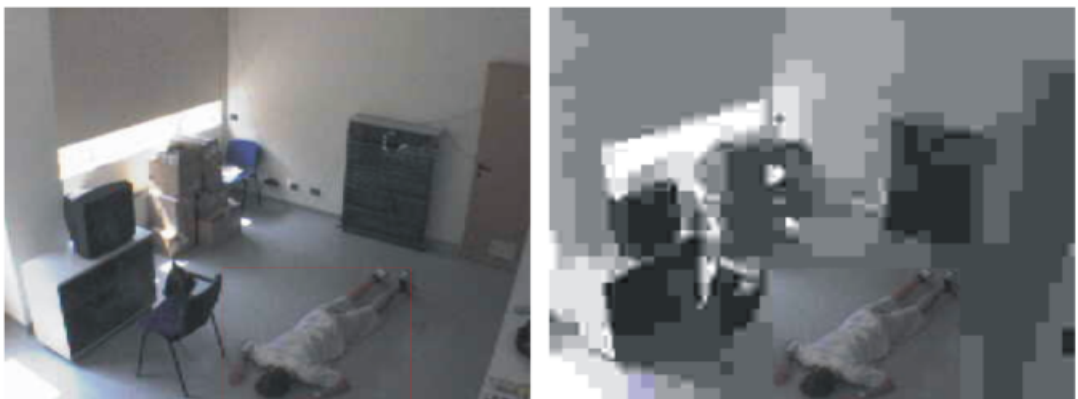
Figure 5: Example of transcoded video: left, original uncompressed frame; right, semantic-based video adaptation in which the fallen person is sent with higher quality to allow identification.
